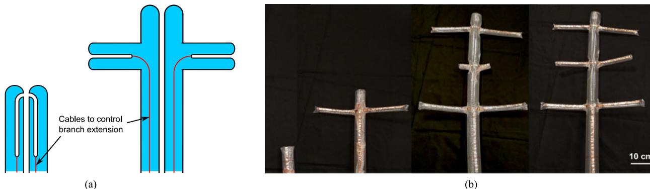
Fig. 7. Tip-extending soft robotic Yagi-Uda antenna. (a) Schematic showing the deployment of branched material and the method to control branch extension through cables attached to the tip of the branch internally. (b) The robotic Yagi-Uda antenna model is sequentially deployed allowing reconfiguration of antenna characteristics as additional dipoles are extended. The center dipole is initially kept from extending, then allowed to extend showing reconfiguration possibilities.
