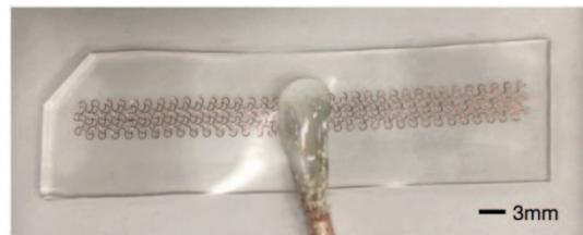
Fig. 8. Fabricated stretchable dipole antenna.
