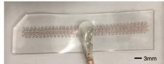
Fig. 8. Fabricated stretchable dipole antenna.
